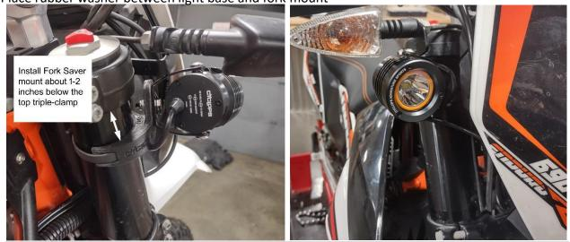
**4.** Once the mounting location is determined, cut the heat-shrink tubing to length, and then heat the heat shrink tubing around the clamp, this prevents the metal portion of the clamp from contacting the metal fork tube.
